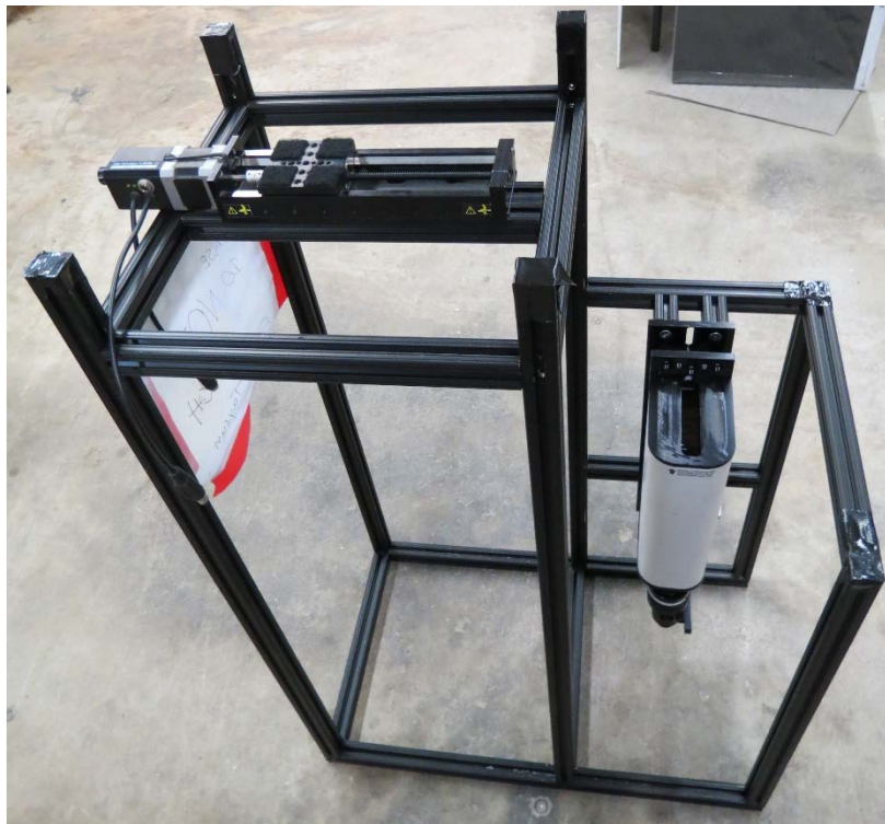
Figure 2. The assembly of a linear stage for the CCD camera with the laser collimator.
