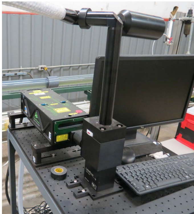
Figure 1. Nd:Yag Laser (power unit not shown) with the laser guide arm attached to the laser emission port.
