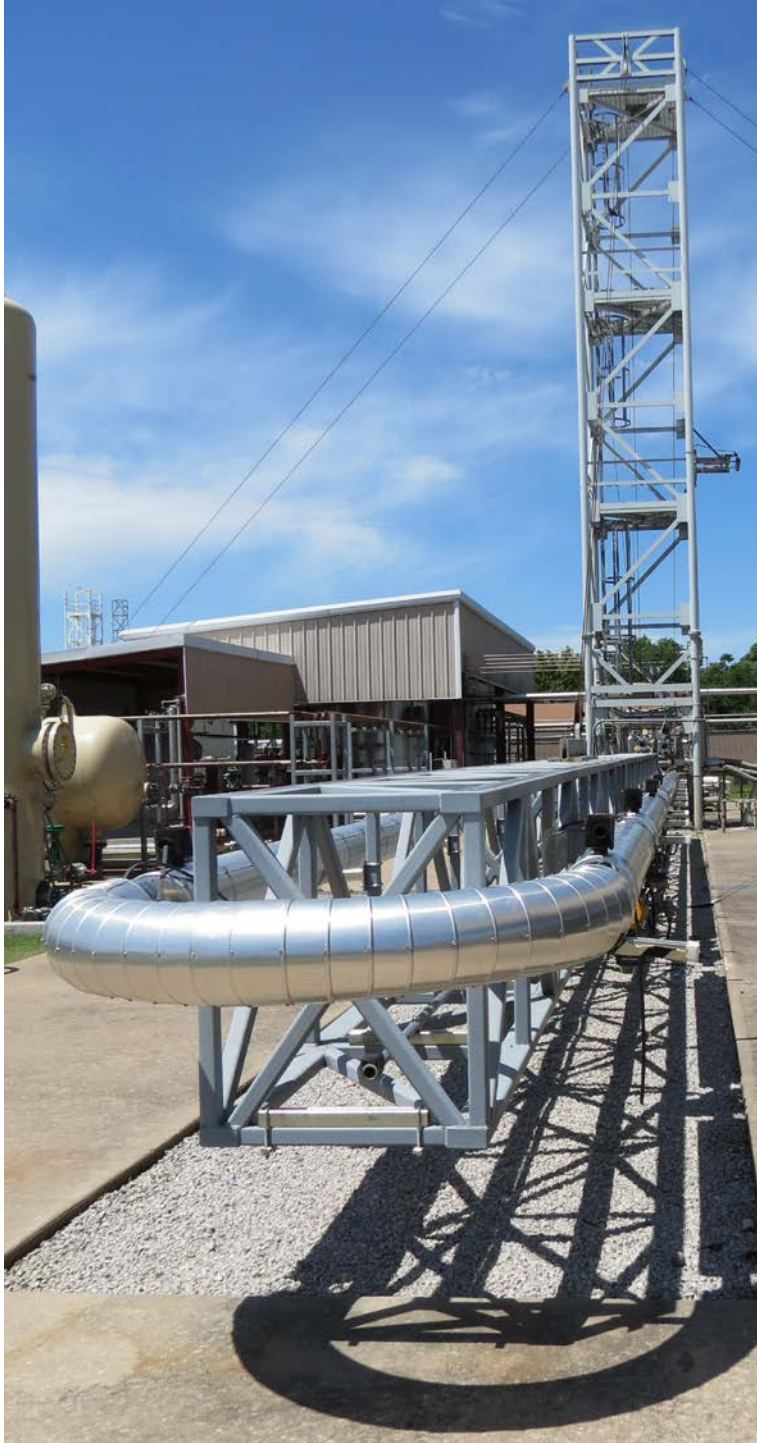
Figure 3. View of 3-in. High Pressure Large-Diameter Gas/Water/Oil Flow Loop
