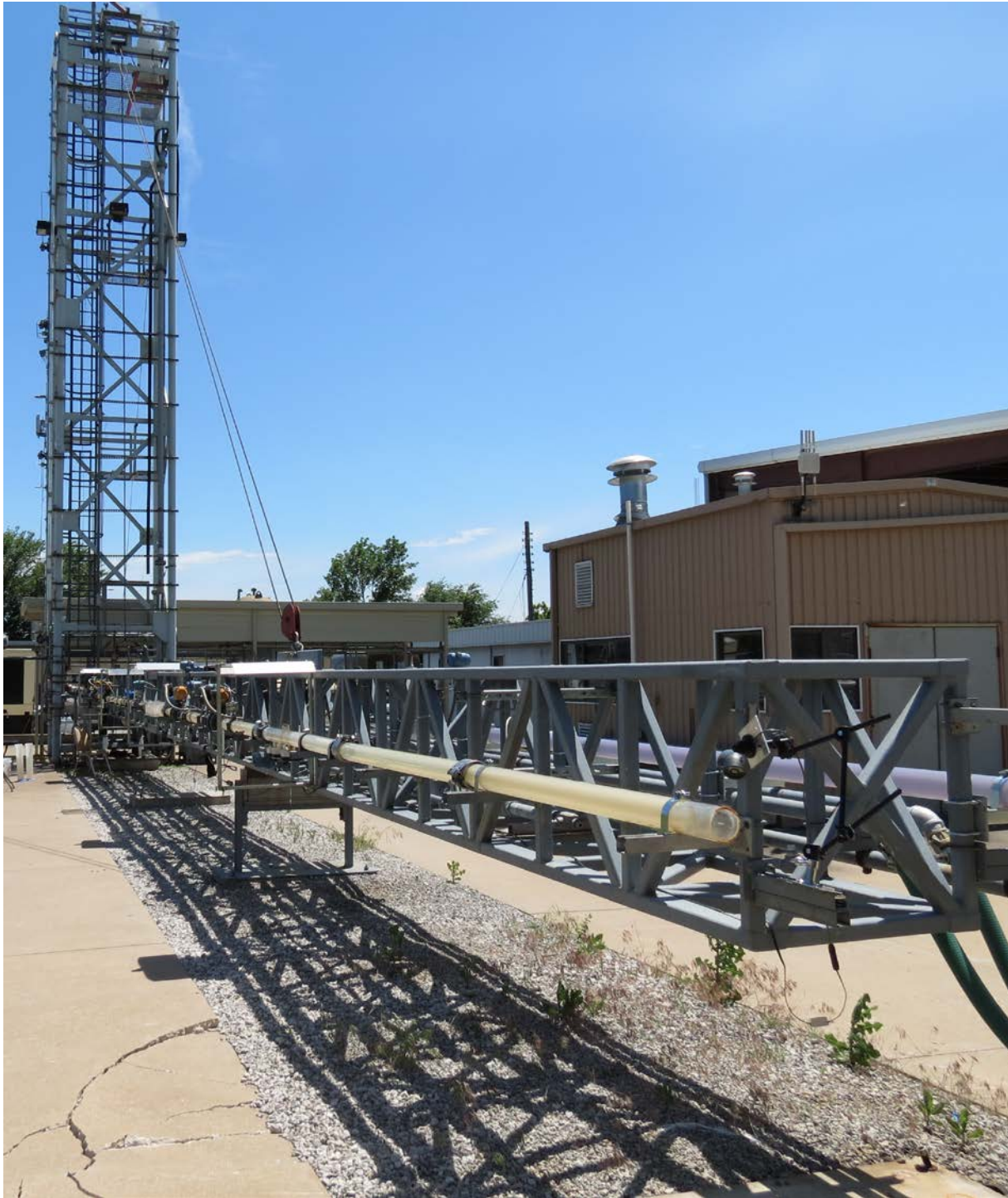
Figure 3. View of 3-in. Gas/Oil/Water Flow Loop
