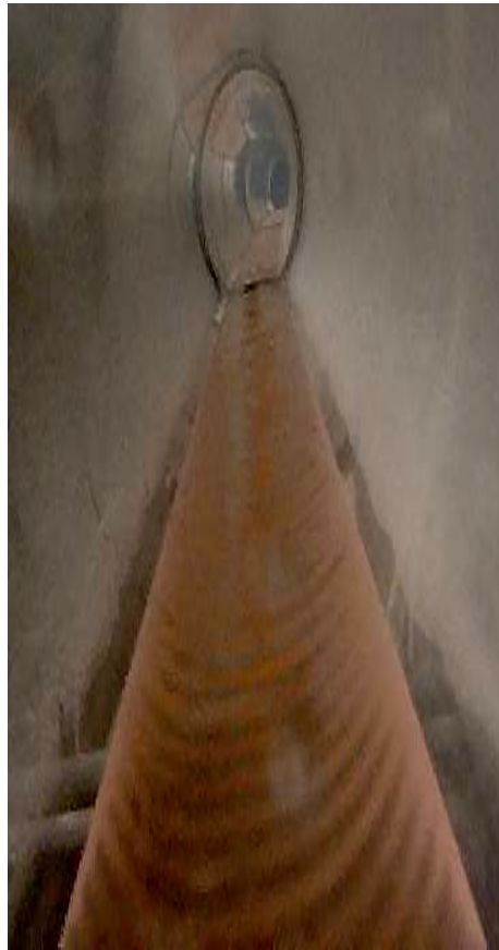
Figure 3. Interfacial waves observed for the two-phase (MEG/Air) flow in a 6-in. ID, horizontal pipeline. Photograph is taken with BIP2 installed within the pipeline facing the flow.
