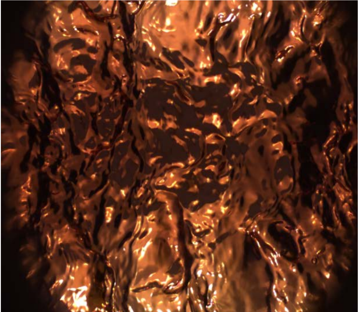
Figure 4. The interfacial waves observed for the two-phase (Mineral Oil/Nitrogen) flow in a high pressure, 6-in. ID horizontal pipeline. Photograph is taken from the bottom of the pipe using Photron SA3 in the Canty Device.
