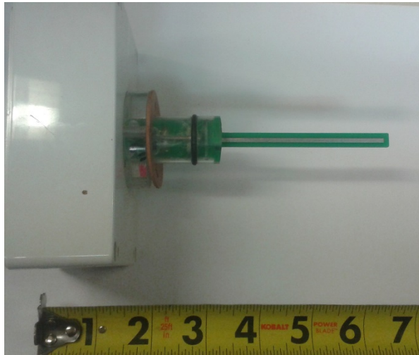
Figure 2. Sensor of a capacitance probe manufactured at the University of Tulsa.
